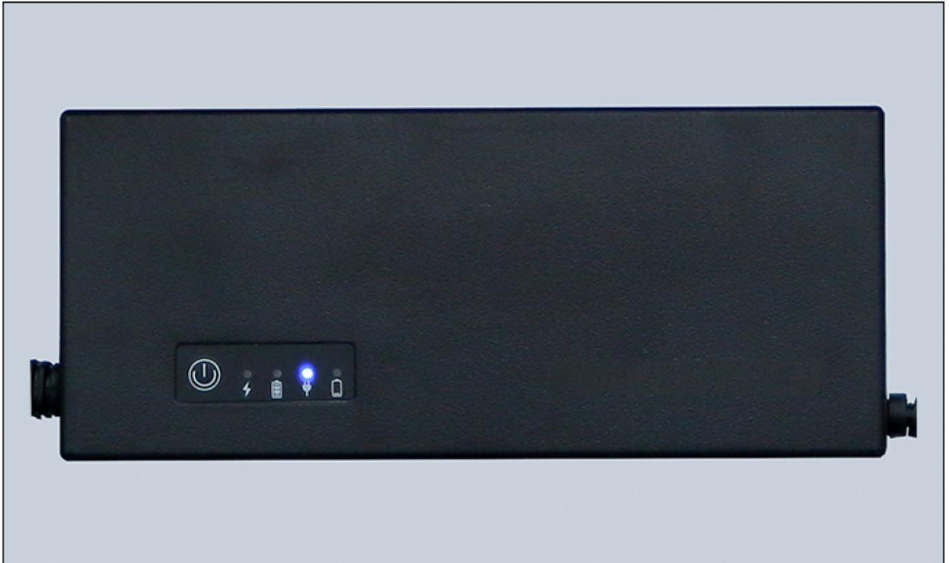
An uninterruptible power supply (UPS) ensures the datalogger continues to record data and transmit alarms during power failure events. The UPS is a DC-DC type, with an integral lithium-ion rechargeable battery. Its input is 12 Vdc, which comes from a mains powered power supply, and its output is 12 Vdc, which is used to power the datalogger and control system.
