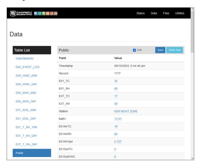
The Data page enables data tables stored in the datalogger to be viewed and downloaded. On some datalogger models\* this page also allows selected fields to be graphed in realtime. It can be selected by clicking on Data on the header/menu bar at the top of the page.
