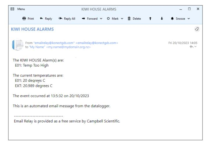
The datalogger can send alarm email messages advising users of events occurring at the station that need prompt attention. All messages are in the same format which is designed to alert users by the subject line alone, with more information contained in the message body. The format is designed to ensure messages are readily identified in a users email In-Box even on the smaller screens of mobile phones. A sample email message is shown above.
