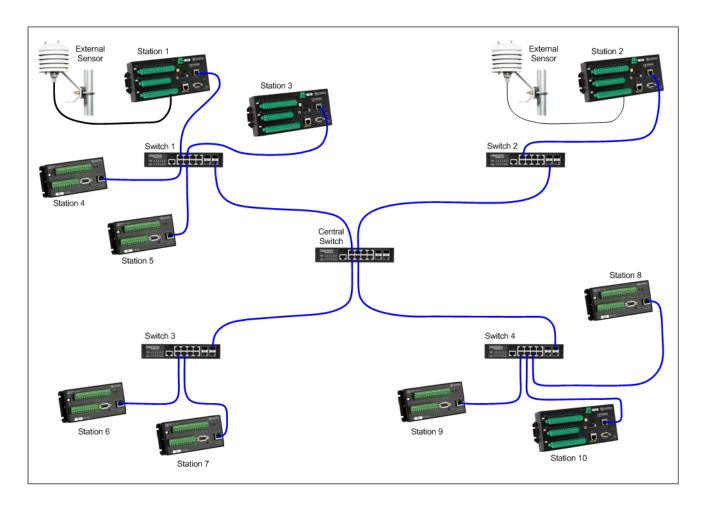
A good design technique is to keep communications between stations localised, as much as possible, to the network switches they are directly connected to.
