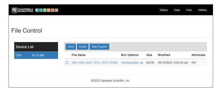
The File Control page enables management of the datalogger files. Files can be sent, deleted, activated, and deactivated. The files page can be selected by clicking on Files on the header/menu bar at the top of the page.
