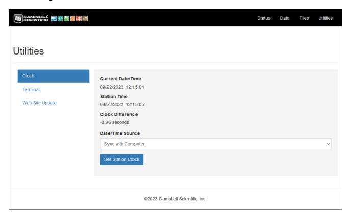
The Utilities page enables setting the datalogger realtime clock and it provides a terminal function. It can be selected by clicking on Utilities on the header/menu bar at the top of the page.
