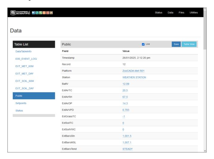
The Data page enables data tables stored in the datalogger to be viewed and downloaded. On some datalogger models this page also allows selected Public variables to be graphed in realtime. It can be selected by clicking on Data on the header/menu bar at the top of the page.
