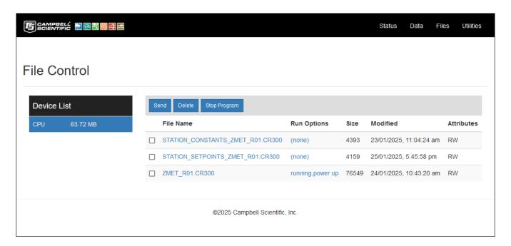
The File Control page enables management of the datalogger files. Files can be sent, deleted, activated, and deactivated. The files page can be selected by clicking on Files on the header/menu bar at the top of the page.
