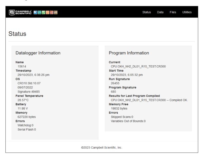
The Status page gives key information about the datalogger and the program that is running in the datalogger. It can be selected by clicking on Status on the header/menu bar at the top of the page.
