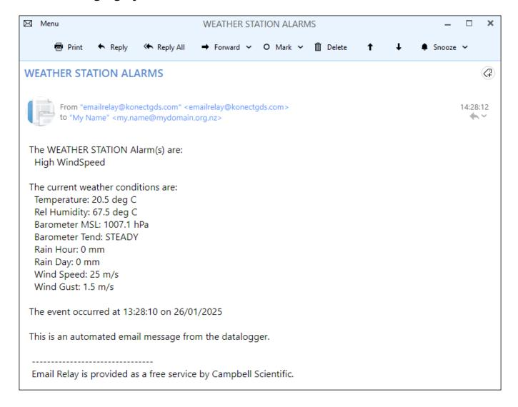
The datalogger can send alarm email messages advising users of events occurring at the station that need prompt attention. All messages are in the same format which is designed to alert users by the subject line alone, with more information contained in the message body. The format is designed to ensure messages are readily identified in a users email In-Box even on the smaller screens of mobile phones. A sample email message is shown above.
