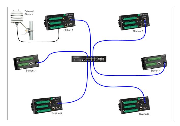
In this example, assuming the PakBus address and the IP address for each station is the station number in the diagram above, the configuration settings would be:
